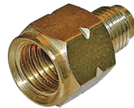
Male 1/4 SAE/7/16" - 20 x Female 1/2 ACME (LHT) Tank Adapter 5713
